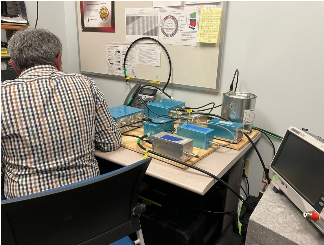
The plywood bases hold the hexaplex Antenna Multiplexer and its various bandpass filters, most using the VA6AM designs. These were much better organized this year.
