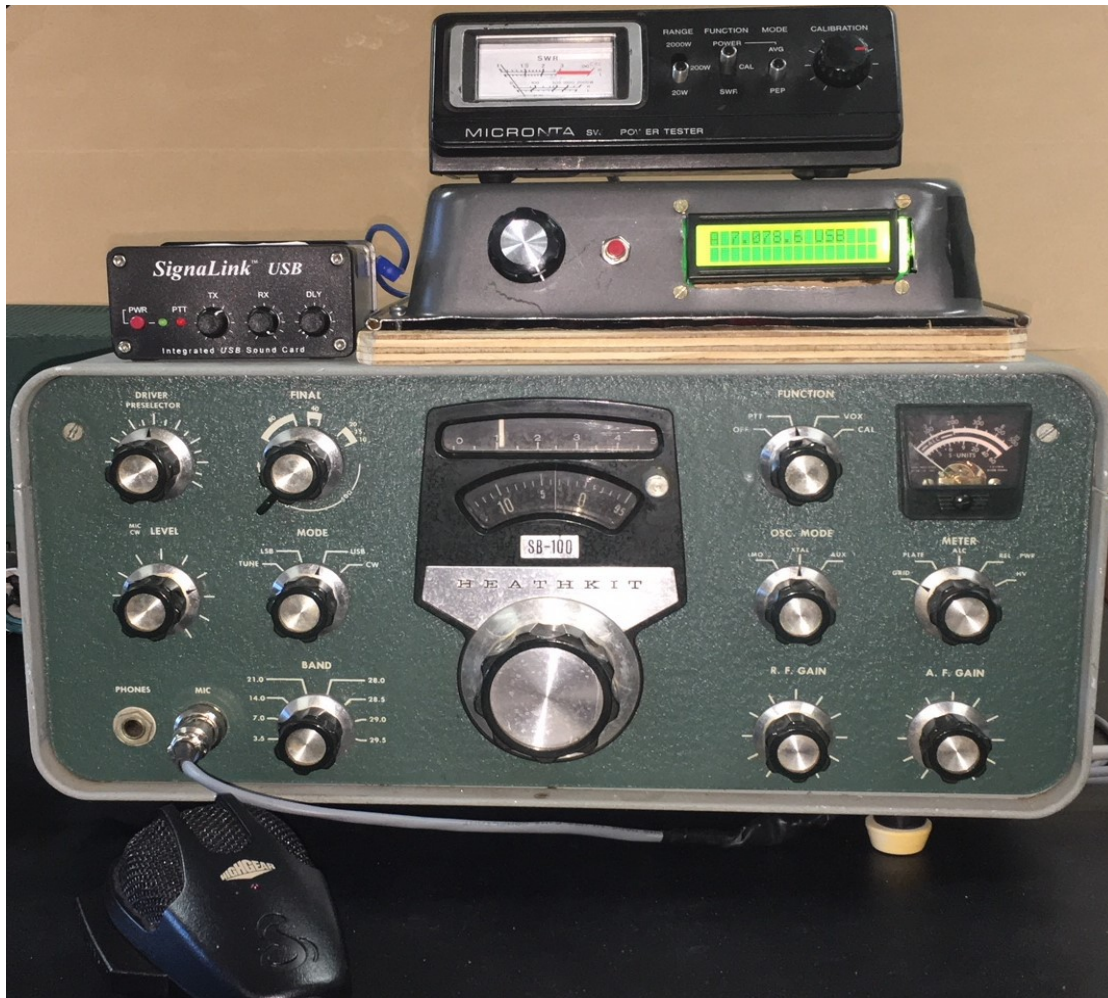
Figure: A digitally synthesized external VFO for older transceivers such as Heathkits build around the HFSIGNALS Raduino with incredible accuracy, computer controllability and additional features over the original internal VFO.
