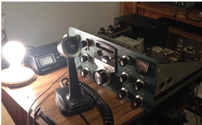
Figure. Excellent power output from a refurbished Heathkit SB-series SSB transceiver.
