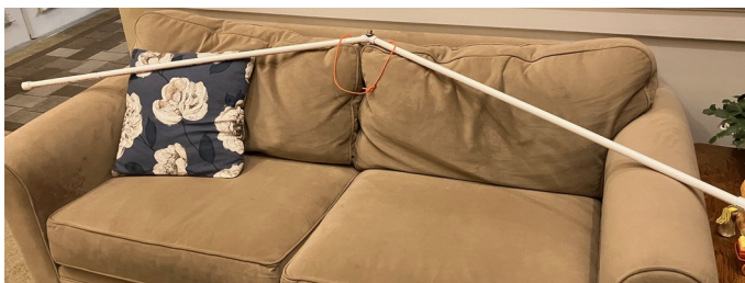
Figure: 6 meter PVC-supported semi-inverted vee antenna, only slightly wider than a traditional living room couch.
