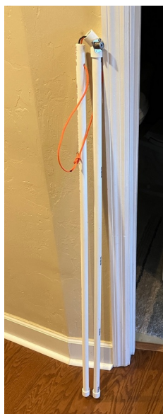
Figure: 6 meter PVC-supported semi-inverted vee antenna, only slightly wider than a traditional living room couch.
