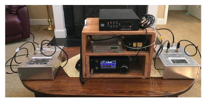
In the photo above, the bypass switch box and VOICE receive only filter are to right of the 7300 station. You can see the two connections of the filter to the connections of the bypass switch box, which are plainly marked.
