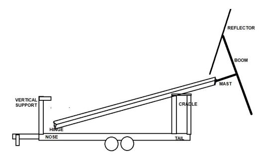
**This requires at least two people.** The torque is excessive for one person to manage. One person can be on the ground stabilizing the boom, while the other on the ladder loosens the nuts with a 13 mm wrench and then removes the boom from the mast.
