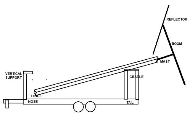
Installation of the MAST with the REFLECTOR High. This is done because with just one element, the boom and one element can be more easily manhandled by two volunteers. One will have to be on a ladder and is at a disadvantage. Their ground helper can greatly stabilize the assembly. (In this drawing, the reflector is supposed to be looking parallel to ground.....)
