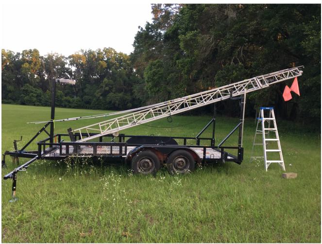
Storing the Elements without having ti disassemble them. Note raised up to avoid being damaged by the edge of the higed base. Centered, within the "yoke" so they can't be crushed by the truck gate.
