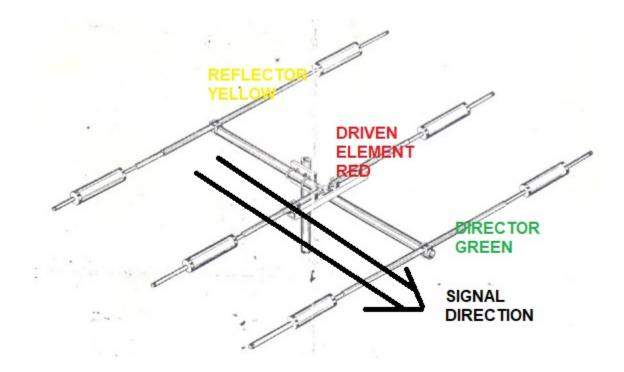
Each element has colored tape to show where it goes. Older tape markings may still be present that had the driven element on the wrong side. Newer tape on the DRIVEN ELEMENT is RED and there is RED tape on the boom where it should go.
