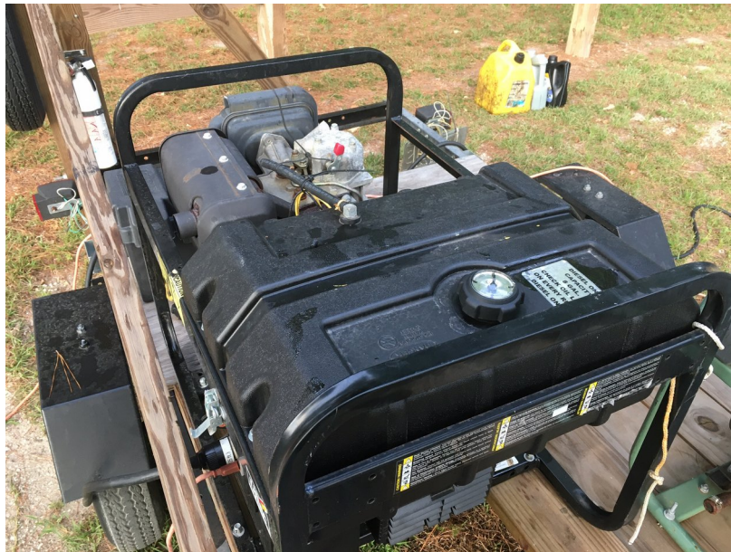
5kW Diesel generator
