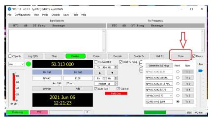
□ With the 7300 set for 100 watts nominal output, Adjust the modulation level so that the 7300 output power level = approx 80 watts, or 80% shown on the 7300 output power measurement. (You can adjust the 7300 output power in real time while sending a tone.) In FT8/FT4 from then on your power will remain pretty constant. The ALC display should show little to no ALC in use with these adjustments.
