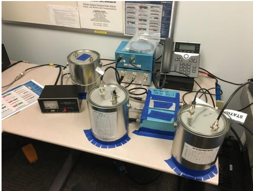
Our collection of Quinplexer (two boxes, back) plus three Butterworth homebrew filters (paintcans) and three VA6AM kit-built bandpass filters. Toward the end of the operational period, a capacitor self-destructed in the 15-meter paintcan filter.
