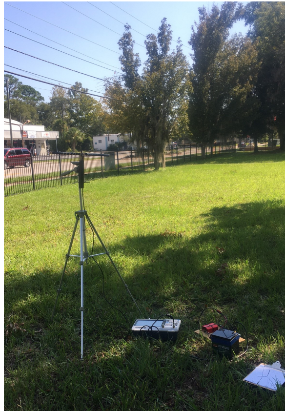
Figure 9: RF background measurement equipment, including Siglent Spectrum Analyzer, standardized test antenna, battery and inverter power supply.
