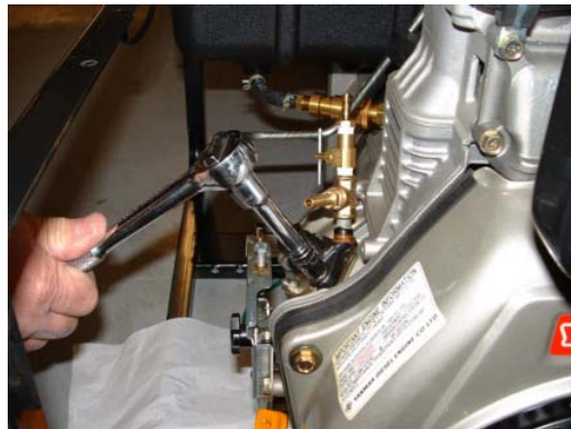
Figure 4-10. Free Injector Pump Piston – Removing Nuts/Cover Plate from Injector Pump
