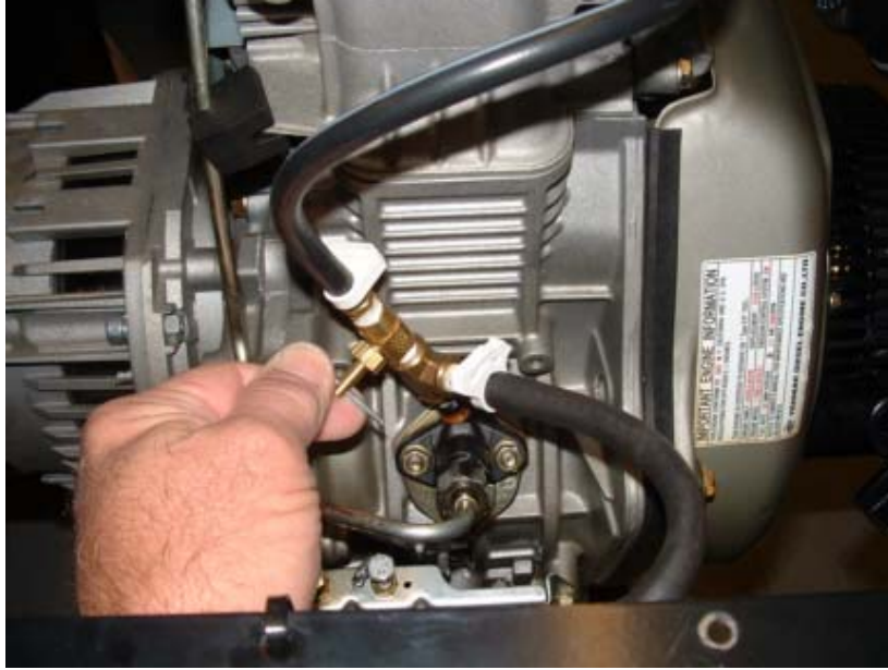
Figure 2-1. Initial Starting Procedure – Opening Bleed Valve
