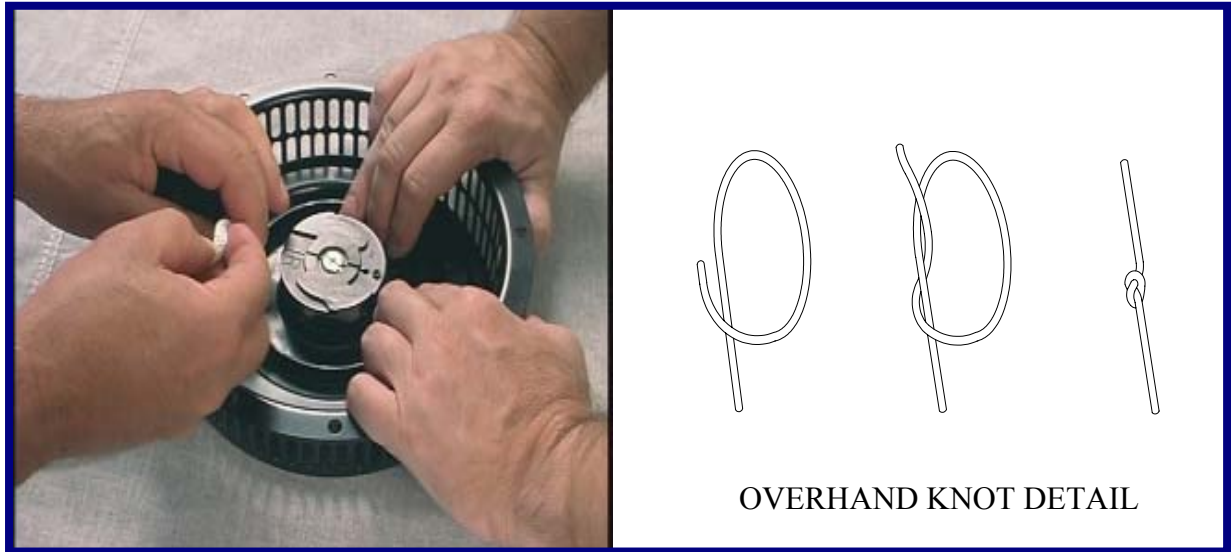
Figure 4-5. Recoil Starter Replacement – Knotting Rope
