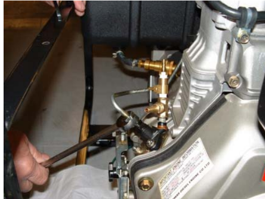
Figure 4-9. Free Injector Pump Piston – Removing Rigid Fuel Line
