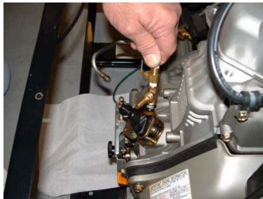
Figure 4-11. Free Injector Pump Piston – Removing Fuel Injector Pump
