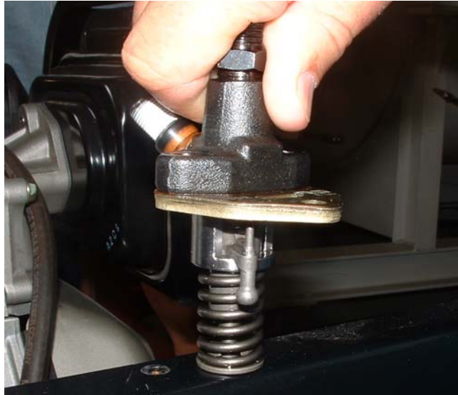
Figure 4-13. Free Injector Pump Piston – Free Piston
