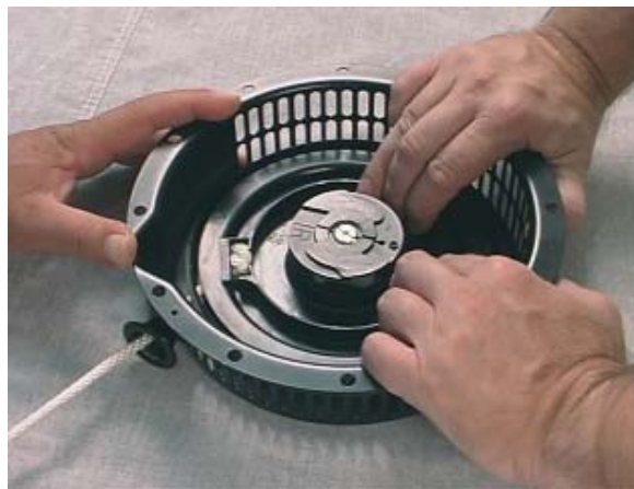
Figure 4-3. Recoil Starter Replacement – Aligning Rope Access
