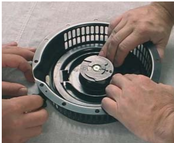
Figure 4-4. Recoil Starter Replacement – Feeding Replacement Rope
