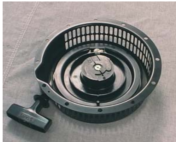
Figure 4-6. Recoil Starter Replacement – Recoil Replacement Rope
