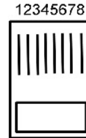
Figure 2-3 Top View (pins visible) numbering of the RJ45 plug pins.
