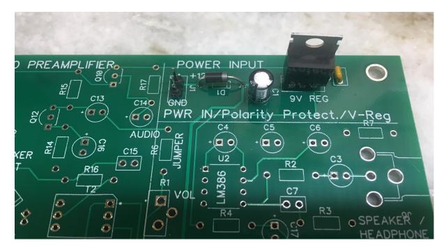
Soldering D1: Be certain that the CATHODE END (the banded end) is toward C1, not toward the J1 power input connector.
