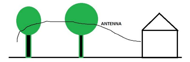
Because this is a receiver and not a transmitter, the antenna requirements are much simpler. The simplest antenna is to stretch 30-100 feet of wire AWAY FROM POWER LINES between outdoor trees or other supporting structures, and slip the wire underneath a window to the radio a few feet from the window.
