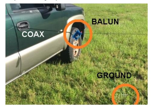
4 A test setup looked like the photo here and gives you an idea of how to utilize this antenna.
