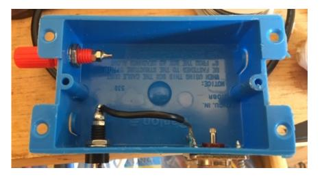
7. Now make your solder connections from the Toroid. The longer end of the white wire goes to red banana plug. The shorter side of the white wire solders to the ground wire from the SO-239. The Red wire solders to the center connection of the SO-239.
