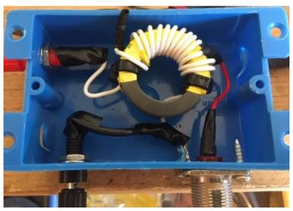
8. Wrap the soldered connections with **electrical tape** to avoid unwanted shorts
