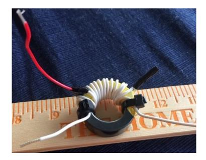
6. Make a solder connection from the ground side of the SO-239 to the black banana plug. Leave approximately 3/4" of bare wire at the SO-239 end, so that you can connect the short end of the toroid white wire to this.
