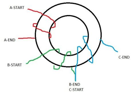
In this drawing, the non-center-tapped winding is "A" and it has a *start* and *end*.
