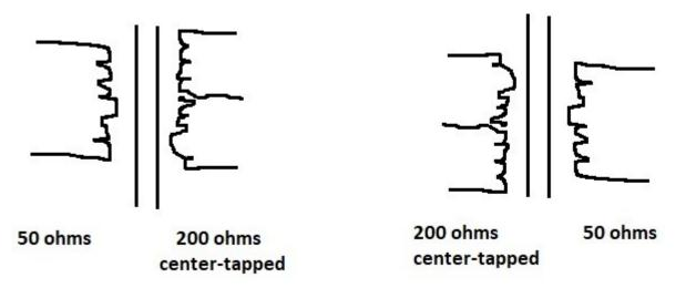
The lower-impedance side has 10-13 turns and the higher-impedance side has 20-26 turns, depending on how many "fit" on your toroid.
