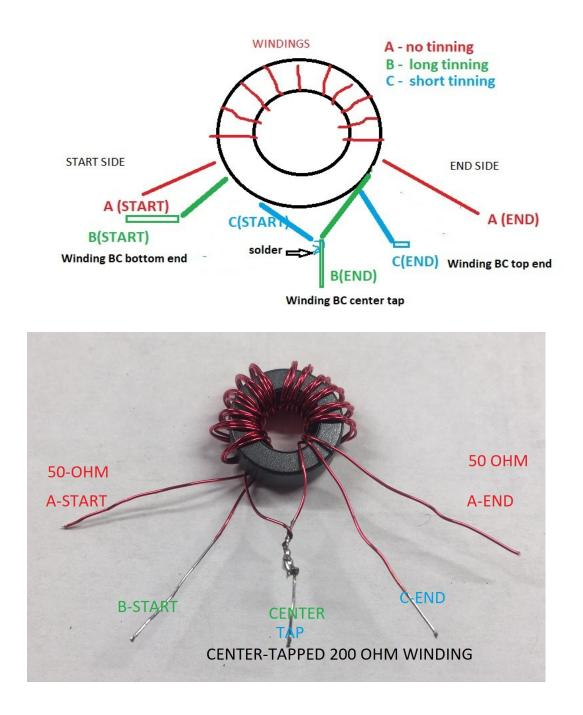
We can now use this type of transformer as either a step-up (with a center tapped secondary) or a stepdown (with a center tapped primary) impedance transformer. See the drawings below:
