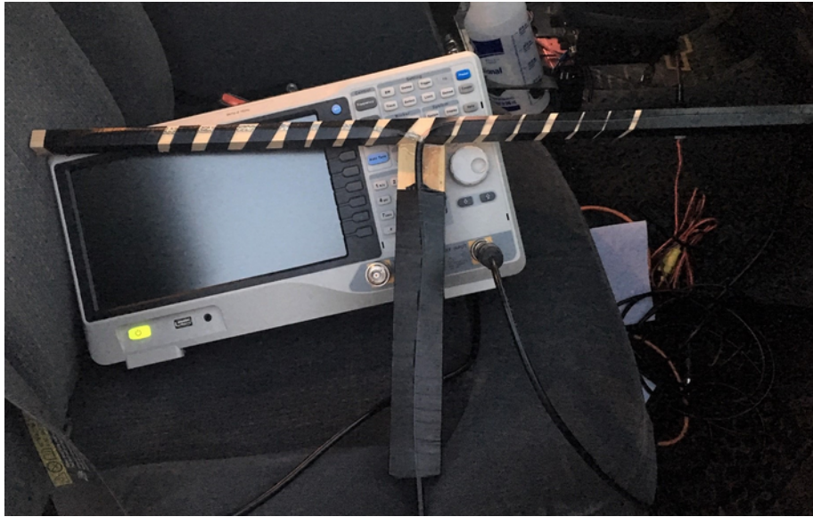
Fig. 1: Simple home-made test antenna for HF measurements.
