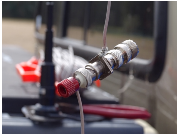
Homemade 2 meter antenna constructed on the fly to overcome one of the Injects
