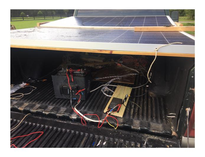
2 Solar Panels Secured to Pickup Truck, combined power approx 500 watts. However our MPPT controllers were only able to take advantage of approximately half that power due to temperature limitations. This could be improved with larger MPPT controllers.
