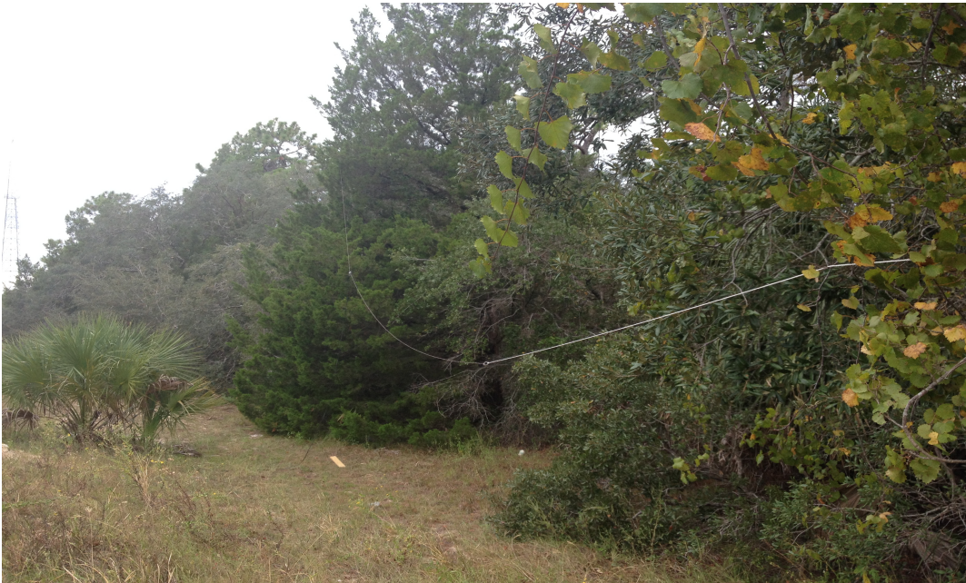
HF Dipole Antenna between trees at Comm Unit #4
